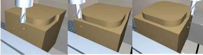
Figure 3 Work-piece updating during the geometric simulation.
